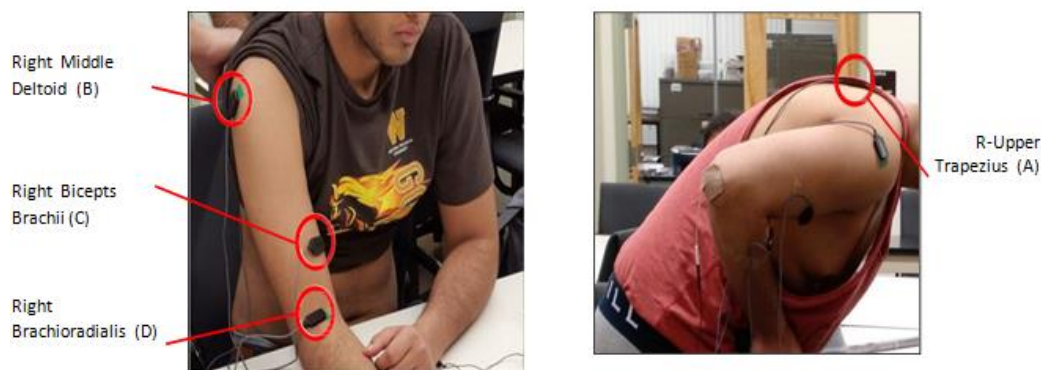
Figure 3. Illustration of EMG electrodes attached to A-Trapezius, B- Medial Deltoid, C- Biceps Brachii, and D-Brachioradialis
