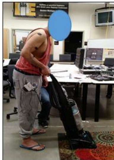
Figure 2. Illustration of a subject performing the task equipped with the upright vacuum cleaner at trunk flexion angle 20^{\circ}
